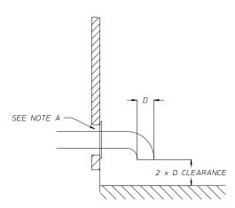
NOTE "A": OPENING MUST BE TWO (2) INCHES (5.08 CM) LARGER THAN DUCT (ALL THE WAY AROUND). THE DUCT MUST BE CENTERED WITHIN THIS OPENING.
